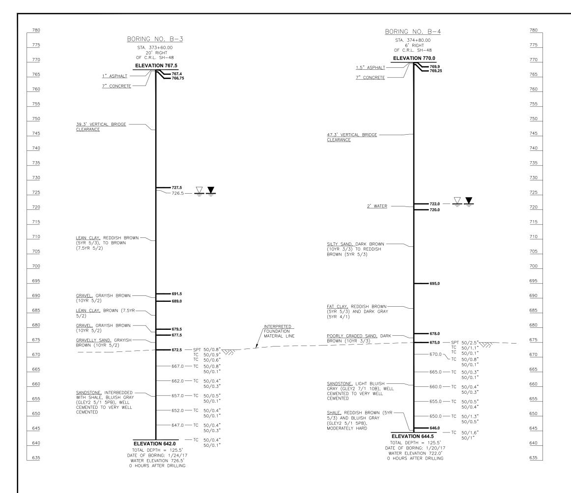
NOTES: SPT DENOTES STANDARD PENETRATION TESTS TCP DENOTES TEXAS CONE PENETRATION TESTS  $\nabla$ DENOTES WATER ELEVATION DURING DRILLING DENOTES WATER ELEVATION AT NOTED TIME DENOTES CAVE IN DEPTH DENOTES ROCK ELEVATION
